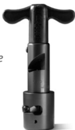
The SCT/QR is a two-piece Cable Prep tool. Part SCT/QR-A cores the dielectric and strips the jacketed aluminum; part SCT/QR-B removes the outer jacket only. The two units are threaded and assembled as one. This feature keeps the tool in a set while not in use and protects the interior parts from damage. Accessory items included with this tool are a 1/8" and 3/32" hex wrench for the set screws and button head screws, a T-bar handle for manual tool use.
